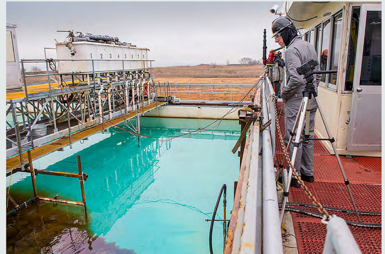
ABOVE: OLEO SPONGE CO-INVENTOR SETH DARLING COLLECTS DARK BROWN OIL FROM THE WATER DURING LARGE-SCALE TESTS.
